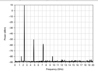
Figure 4. PXIe-5654 with PXIe-5696 Typical Spectrum at 2.4 GHz
