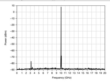
Figure 6. PXIe-5654 with PXIe-5696 Typical Spectrum at 10 GHz
